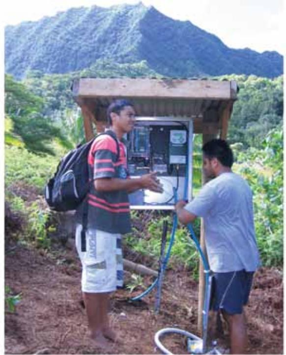
*Avana streamflow station setting up instrument housing, bubble sensor and logging equipment. Note the steep mountains typical of Rarotonga.*
