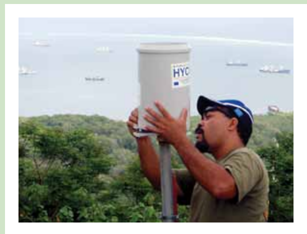
Servicing automatic raingauge on Sokebs Rock above Kolonia
