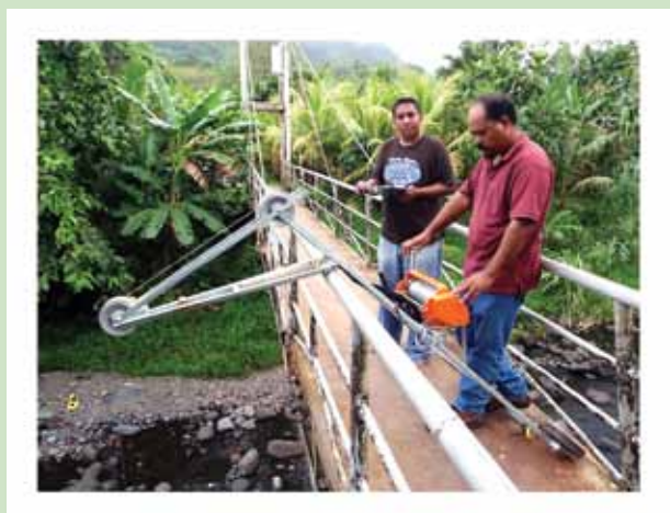
DTCI staff undertaking discharge measurement from the foot bridge at Senipebn
