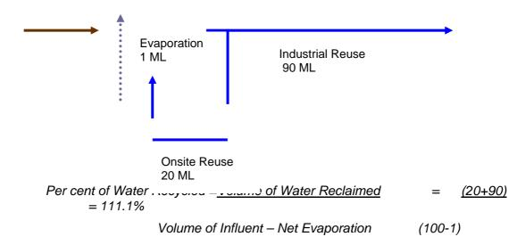
3. Reclaimed water is used on site, supplied for agricultural reuse and supplied for urban reuse through a third pipe system to urban households for toilet flushing and garden watering and for irrigation of open space community facilities.
