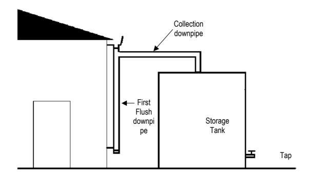
PVC piping and T-joints, widely available and commonly used for standard downpipes, can be used to construct the first flush downpipe.
