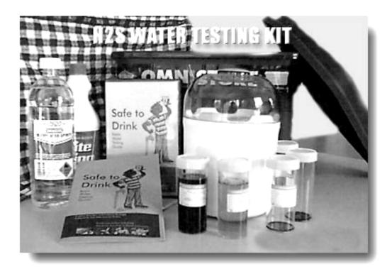
Fig 1. The H<sub>2</sub>S water testing kit
