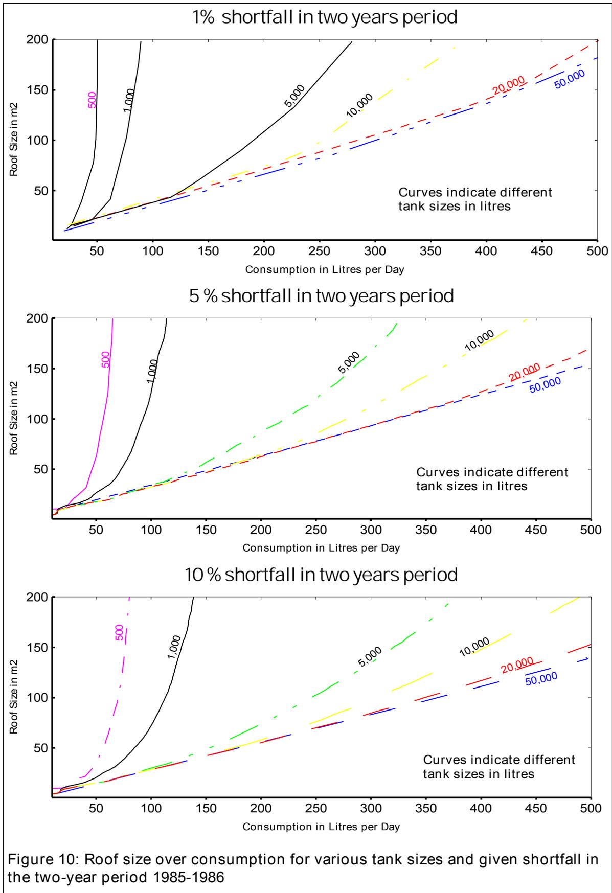
Other information such as determining the possible consumption for a given tank size and chosen shortfall can be retrieved by interpolation between the “tank-curves” in Figure 10.
