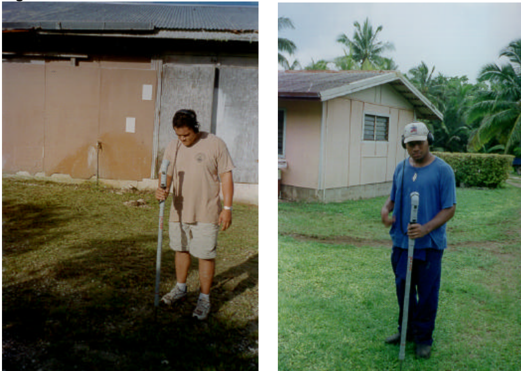
Figure 4: Listening for the generated pulse using the RD-500 PVC pipe detector receiver
