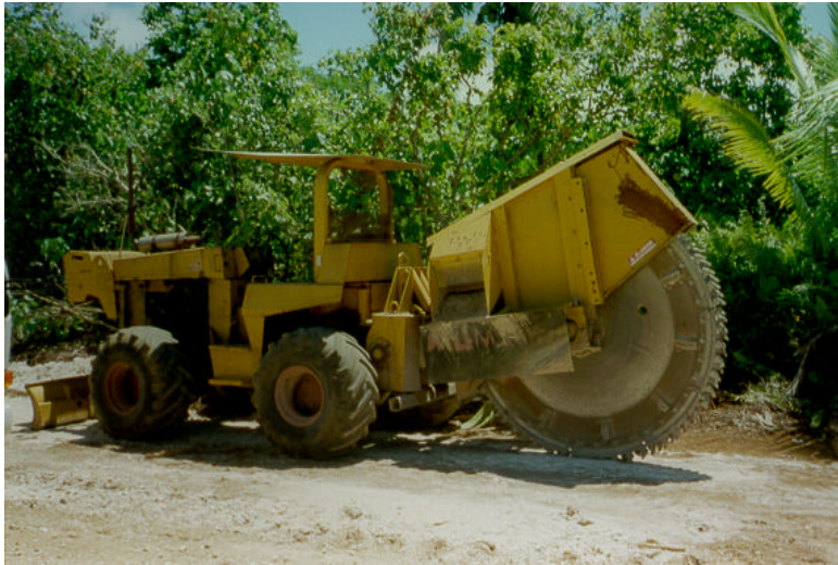
Figure 2: Trench digger used in the laying of pipes and electrical and telephone cables in Niue.
