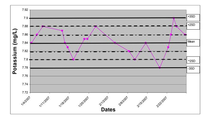
3.7.2 Table 2 outlines the conditions on the control chart that indicate that the method is probably no longer "in control" and actions to check the accuracy and precision should be taken.
