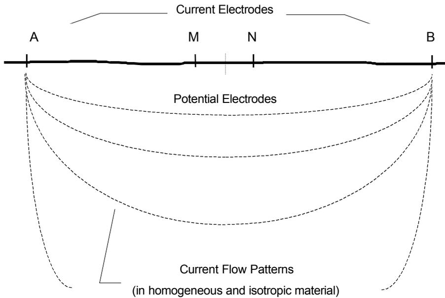
Figure 4: Schlumberger electrode array.  $AB$  distance  $\geq 5MN$  distance
