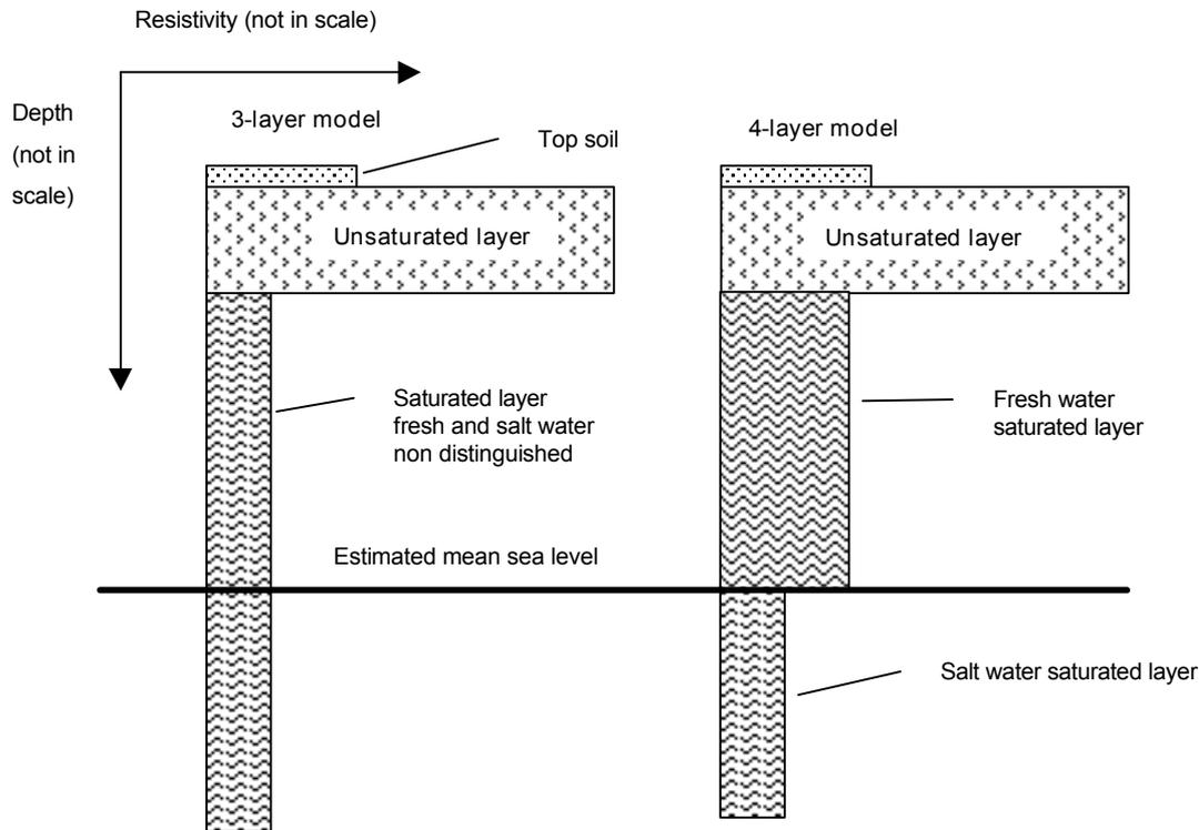
Figure 5: Interpretation of resistivity soundings as a 3-layer model and 4-layer model
