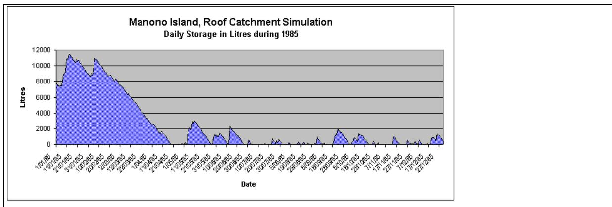
Figure 7: Daily Storage in litres for 1985 in a 19260 litres tank
