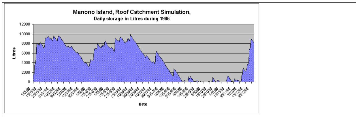
Figure 9: Daily Storage in litres for 1986 in a 19260 litres tank
